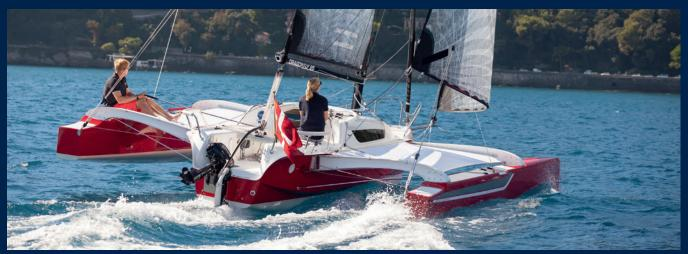
All three hulls in white Gelcoat finish + deck and structural parts of the interior are hand-laid fiberglass and Biaxial fibres combined with Divinycell closed Cell foamcore sandwich construction. Nonskid is part of the deck molding. The 4 wings and the 2 structural Composite bulkheads are made in UD and Biaxial fibres in Vinylester resin and tempered. Collision bulkhead in all three hulls.
