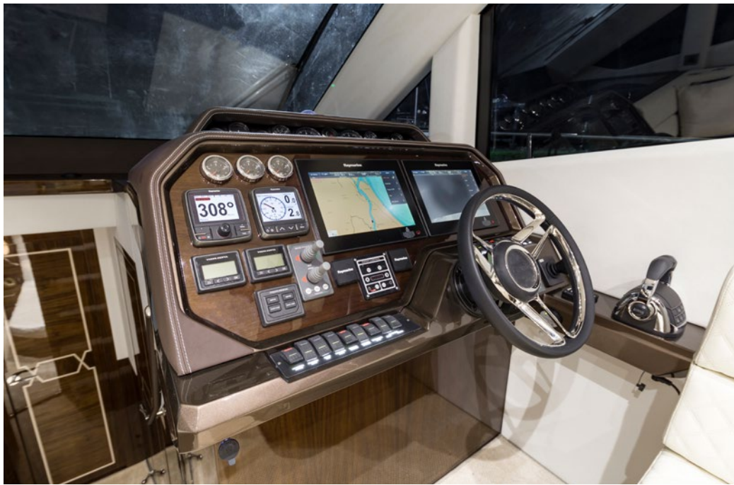
The helm can be fitted with a variety of navigational equipment —
