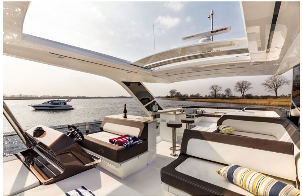
— The carbon bimini top can be opened with a touch of a button
