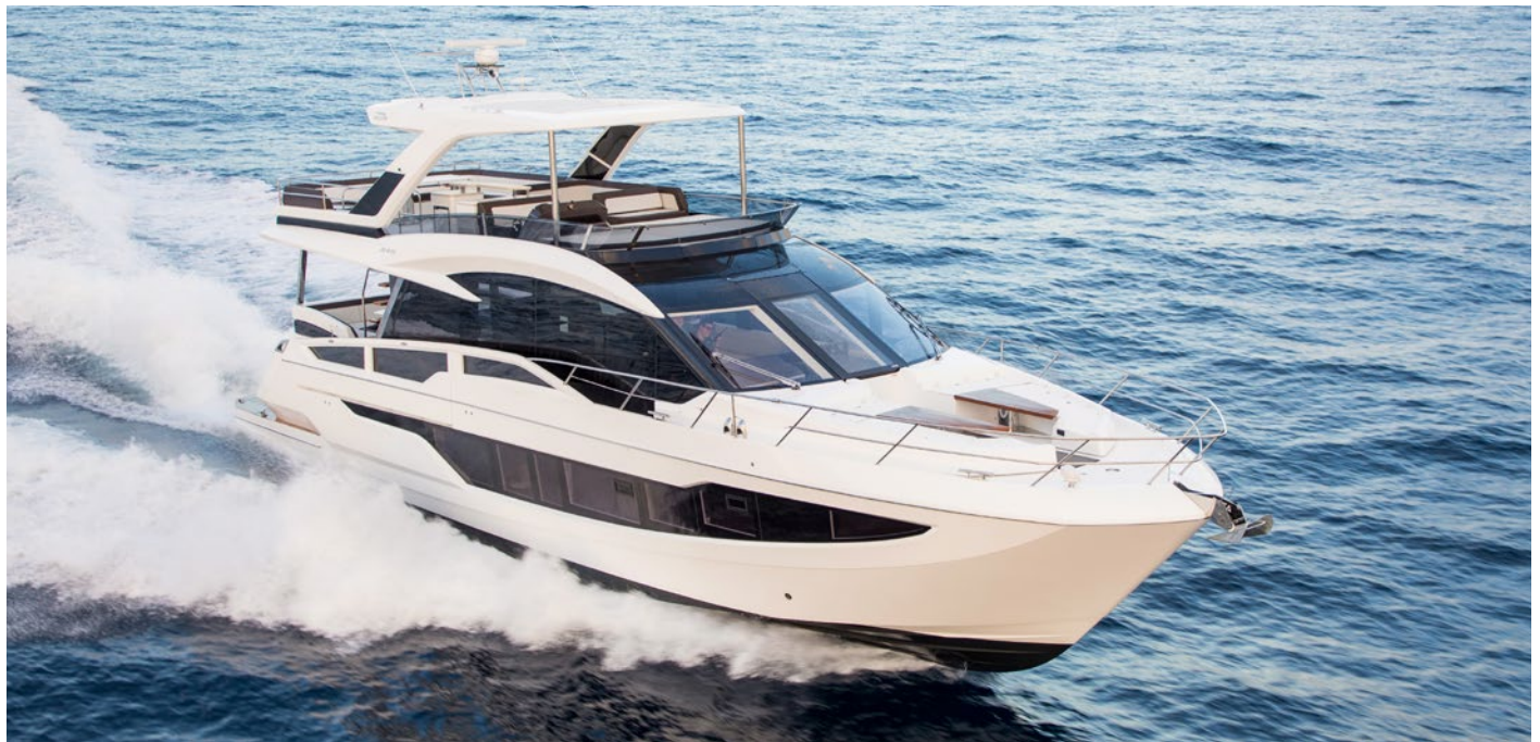
The carbon construction of the top deck and bimini allows for better weight distribution —
